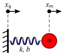
If we consider the ground to be fixed and apply an external force, f, to the 'mass' shown above, the equation of motion is:
